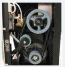
Vertical tensioned belt provides extended life and reduced maintenance costs by eliminating multiple belts that stretch at different rates.
